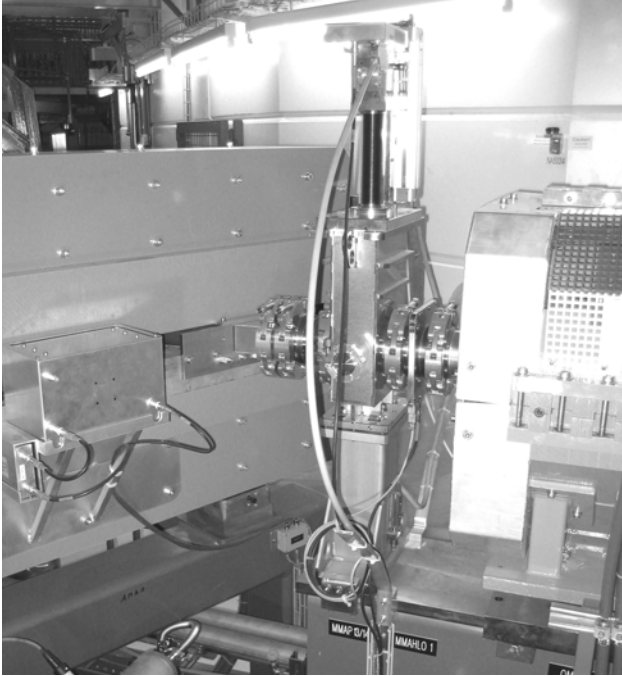
Fig. 4. Thick profile monitor with compressed-air actuator. A beam-line halo-monitor is placed at the right bellow, and an external loss monitor is seen to the left.
