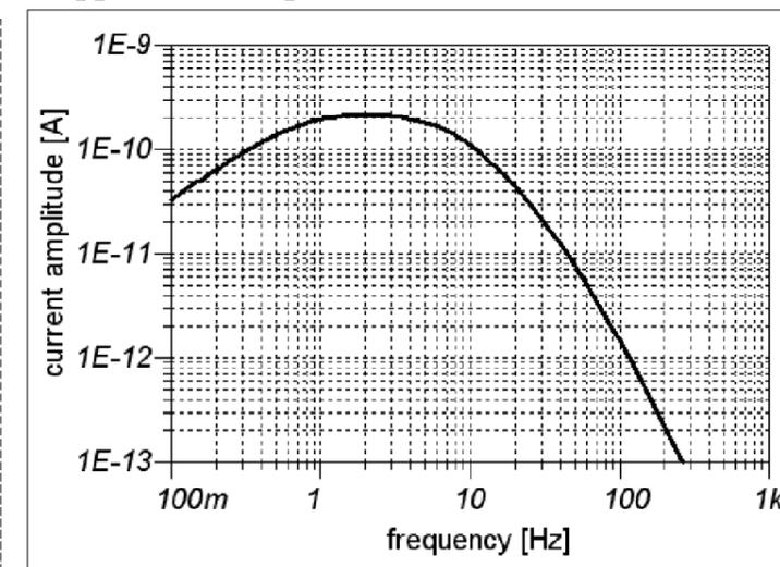
current at read out electronics due to a beam current step
