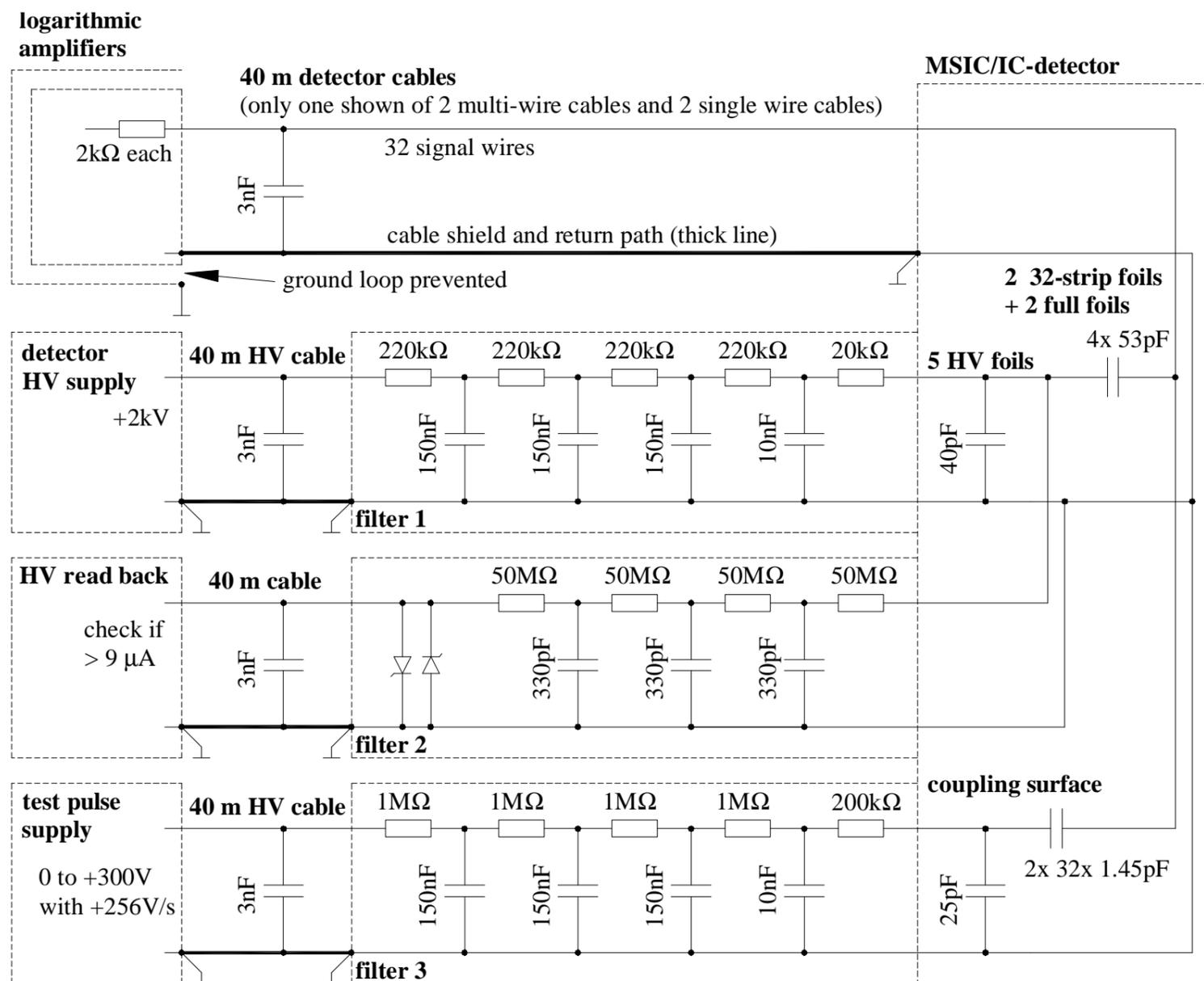
current at read out electronics due to a ripple of 1 V amplitude at entrance of filter 1
