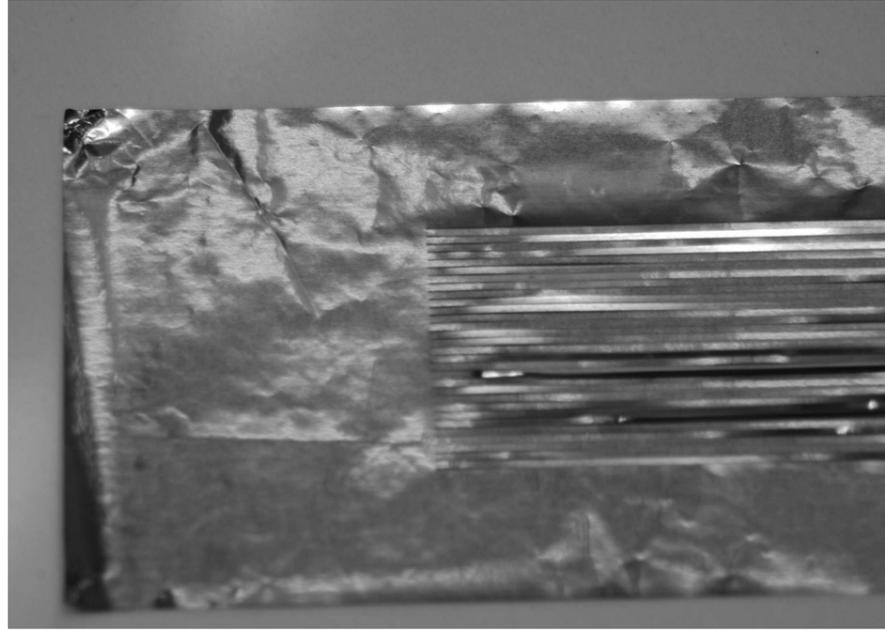
6  $\mu\text{m}$  titanium foil with 1 mm strip pitch
