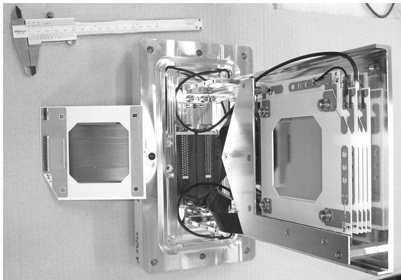
FIGURE 5. Thin profile monitor in front of the degrader. When used as MSIC, it is equipped with a hood with 50 \mu\text{m} titanium windows. Left: a single frame with strip foil.
