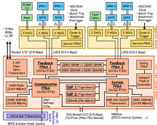
Figure 5: IBFB digital signal processing hardware architecture: PDC board with ADC/DAC mezzanines.
