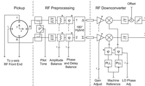
Figure 4: Proposed BPM RF front end (x-axis only).
