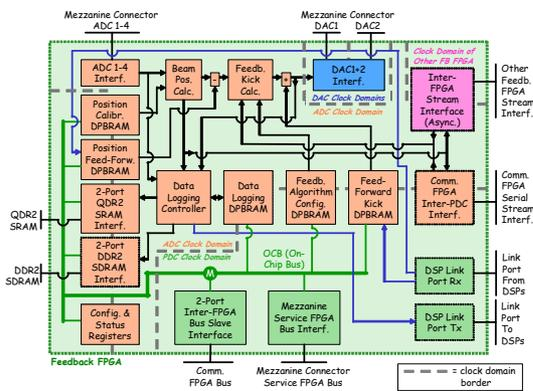
Figure 6: Firmware architecture of the Virtex4-SX “Feedback” FPGA on the PDC board.
