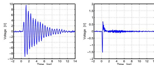
Figure 2: Comparison of beam induced signal at resonant stripline pick-up (left) and button pickup (right).
