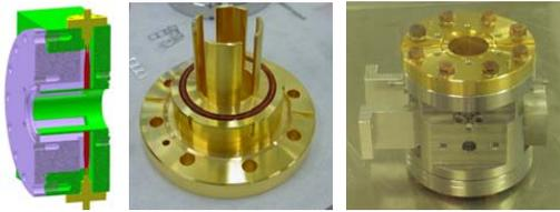
Figure 3: Resonant Stripline BPM Pickup.
