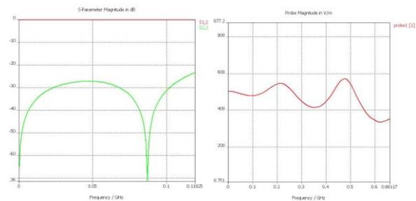
Figure 8: a) Simulated S-parameters (left side) and b) transverse electrical field strength of IBFB stripline kicker (right side).
