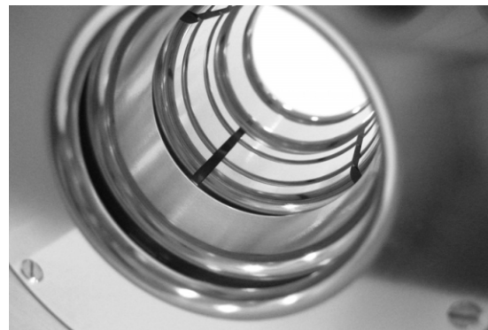
Figure 2: 4-segment ICPM. The electrode configuration from outside to the centre is: ground/high voltage/halo-monitor/position-monitor (= centre electrode). The position monitor covers the full radius of 21 mm, while the halo monitor is fed only from the outer 8 mm. The separatrix splitting the active length of 58 mm between both results from the electric field configuration.
