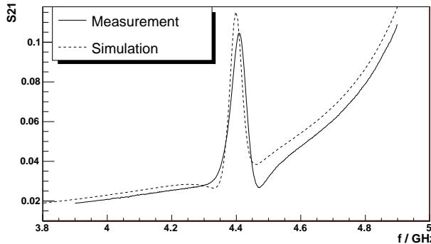
Figure 7: Transmission between orthogonal ports of at FLASH installed BPM without long cables: measurement and simulation (shift of slot position: 0.09 mm).
