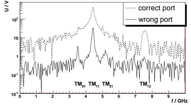
Figure 5: Fourier transformation of signals shown in Fig. 3. Monopole mode leakage at 3.5 GHz is observed too. The first quadrupole mode ( $\text{TM}_{21}$ ) at 5.2 GHz and the second dipole mode ( $\text{TM}_{12}$ ) at 7.6 GHz are visible.
