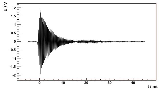
Figure 2: Time domain response signal from reference resonator with visible reflexion after about 14 ns.
