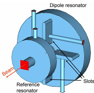
Figure 1: Design view of a cavity BPM, here only the vacuum parts are shown.
