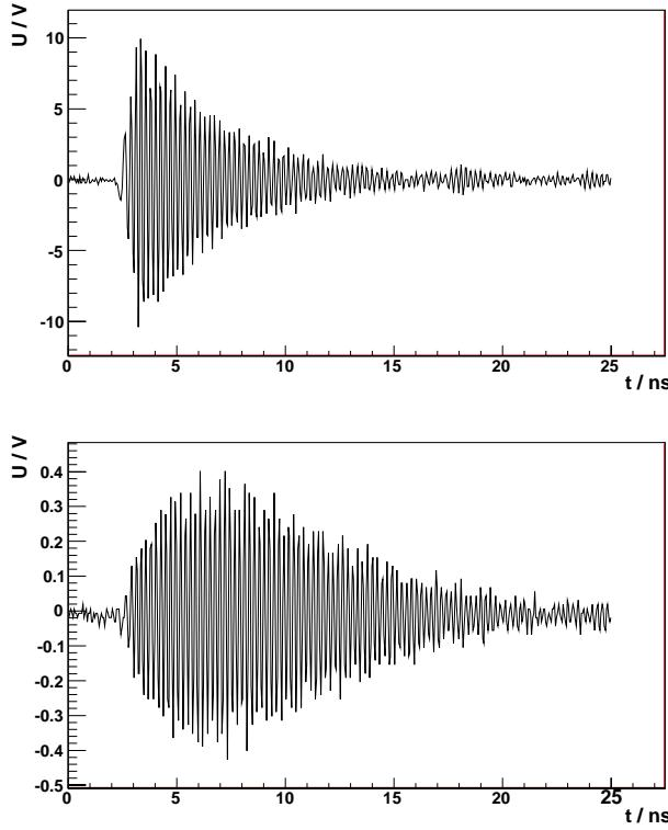
Figure 3: Time domain response signal of dipole resonator. Top: with beam offset of 1.08 mm, bottom: from the orthogonal port. Note the different vertical scales.
