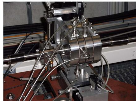
Figure 9: Photo of the installed cavity BPM second generation at FLASH.
