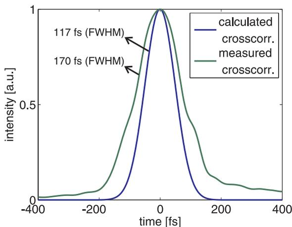
Figure 6: Calculated jitter-free (blue curve) and measured (red curve) cross correlation of the Yb and the Ti:Sa Laser.
