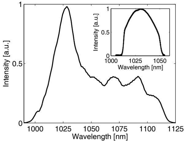
Figure 3: Broad spectrum of the amplifier as used for the EO monitor. Inset: Spectrum of the oscillator
