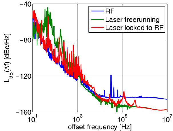
Figure 4: Phase noise measurement of the reference signal, the free running and the locked laser
