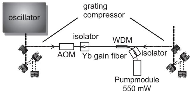
Figure 2: Scheme of the amplifier; AOM, acousto optic modulator; WDM, wavelength division multiplexer
