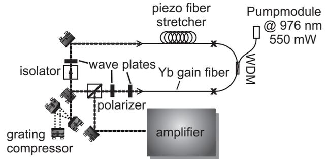
Figure 1: Scheme of the oscillator; WDM, wavelength division multiplexer
