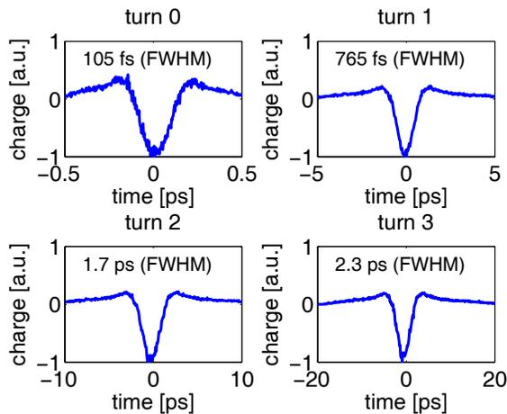
Figure 5: Charge distribution of the sliced bunches from turn 0 to turn 3
