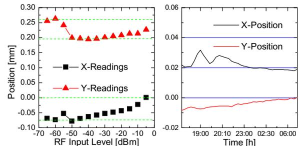
Figure 2a: Beam current dependence of DBPM system. 2b: Long term stability of RF front end. The large movement in x-direction between 18:30 and 20:30 (zoomed out) is due to mechanical deformation caused by heat up while the sun was directly shining on the BPM simulation chamber.
