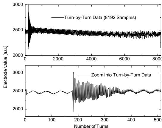
Figure 4: Measurements with DBPM system in turn-by-turn mode. (a) Complete data set from one QDR channel (8192 samples). (b) Zoom into above data (first 500 samples).
