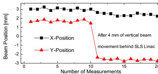
Figure 7: Measurements of DBPM system in pulsed mode performed at SLS linac with single bunches of 1 nC.
