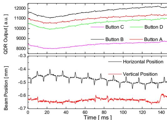
Figure 6: Measurements with DBPM system in closed orbit mode taken at ELETTRA during injection.
