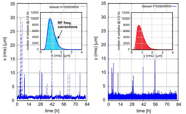
Figure 2: Plot of the RMS values of horizontal and vertical position readings at all 72 BPMs including the histograms of this run.
