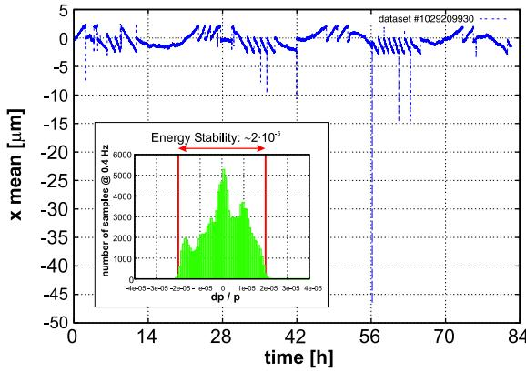
Figure 3: Mean value of the horizontal orbit with respect to the “Golden Orbit” during a 3 days “top-up” run at 180 mA. The proposed frequency correction  $\Delta f$  is applied whenever a threshold of 5 Hz is passed corresponding to an energy deviation  $dE/E \approx 2 \cdot 10^{-5}$ .
