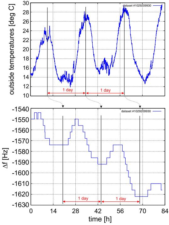
Figure 4: Correlation between the outside air temperature and RF frequency changes during the 3 day user run. With some thermal delay temperature maxima correspond to frequency minima.
