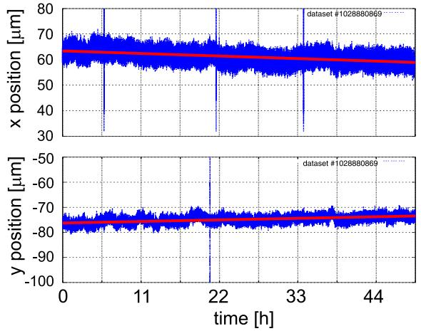
Figure 5: Horizontal and vertical photon beam position at the first X-BPM at the protein crystallography beam-line. The straight lines indicate a daily drift of  $2.3 \mu\text{m}$  horizontally and  $1.7 \mu\text{m}$  vertically.
