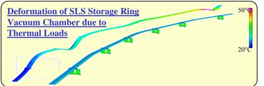
FEA-simulations indicate movements of up to  $2 \mu m/^{\circ}K$  in the transverse plane at the positions of the BPM blocks
