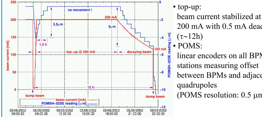
200 mA with 0.5 mA deadband linear encoders on all BPM stations measuring offset between BPMs and adjacent (POMS resolution: 0.5 µm)
